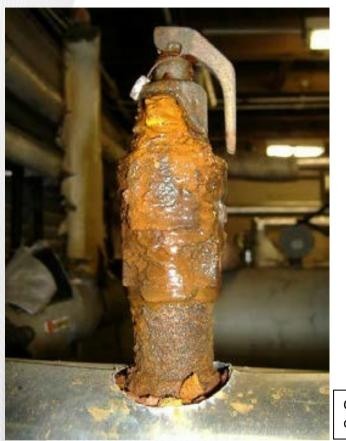
Corrosion caused by damaged diaphragm
