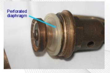
Excessive wear of valve spindle.
