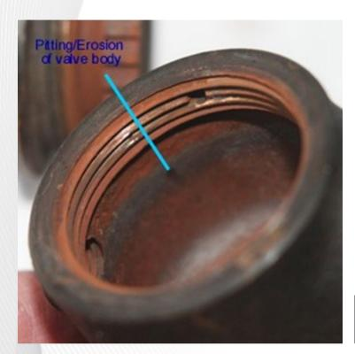
Pitting/corrosion damage on valve body.
